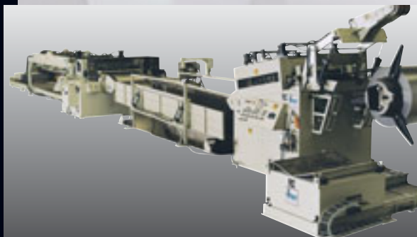
Cut-To-Length Systems 48" wide x .200" thick x 30,000 lb. Cut-to Length system featuring a high capacity 4-roll ServoMax III feed unit. This unit is ideal for CTL applications providing twice the contact area with half the roll pressure which transmits into more accurate blanks.
