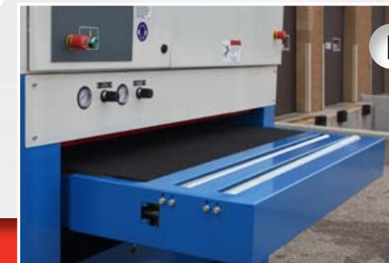
Picture K: Contact drum with barrel brush head which allows for cross/burr removal with superior finish
