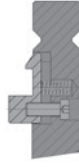
Safety-Click® Applicable for tool weight up to 12.5 kg/28 lbs. (NS I + II + AS II)
